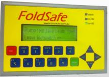
Maximised safety with optimum production Foldsafe uses a beam encoder to do speed and stopping distance monitoring Primary and auxiliary stops ensure safety at all times even if hydraulic valves fail So any valve malfunction will be detected and a pre-warning will be displayed Foldsafe interfaces with both Light curtains or Lazers
